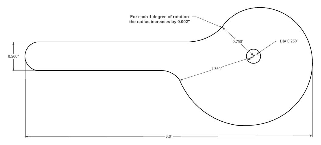
Constructed from Aluminum, two thicknesses 0.25" thick and 0.375" thick
